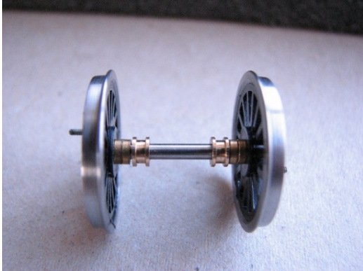
Wheels and bushes assembled on an axle.
