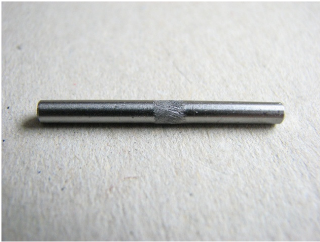
Axle knurled for gear.
